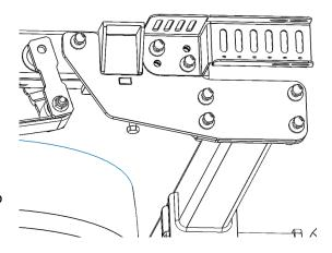
Fit the sensor to the retainer bracket and secure it with the 1x screw, 1x washer, 1x nyloc nut.
