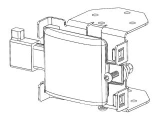
3. Slide the plastic cover over the retainer bracket and loosely secure with 2x screws, and 2x washers.
