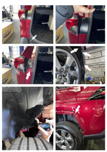
the wheel arches carefully peel the bumper away from the car. (Simultaneously pull up and out sharply and firmly to release the bumper from the car)
