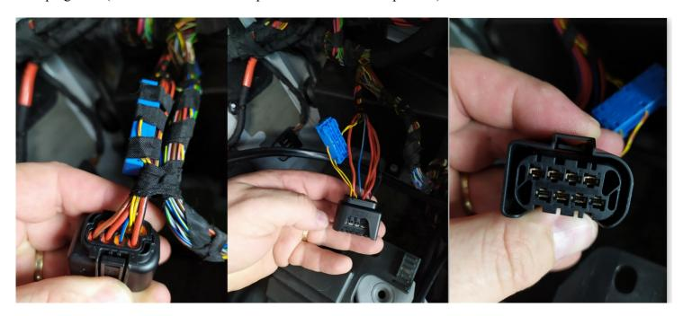
Connect all branches as follows to: Cut out plug and solder wires to
