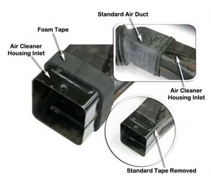
Apply sealant to the inside of the standard air duct and to the outside surface of the pre-cleaner housing outlet, install the standard air duct onto the pre-cleaner housing outlet, secure with the standard hose clamp.
