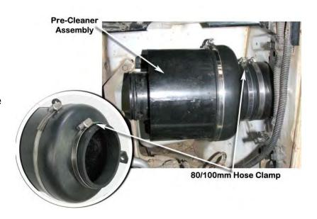
Align the two hoses (items 10 &12) for best fitment, ensure that the snorkel outlet hose (item 10) is installed hard up against the shoulder of the snorkel body outlet snout, tighten the 100/120mm hose clamp (item 15).
