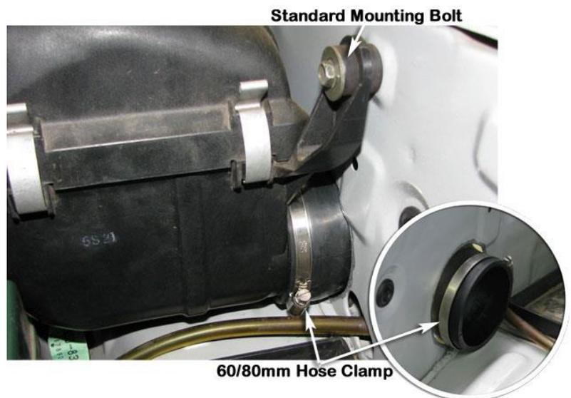
Align the air entry hose (item 10) to the hole in the guard panel.
