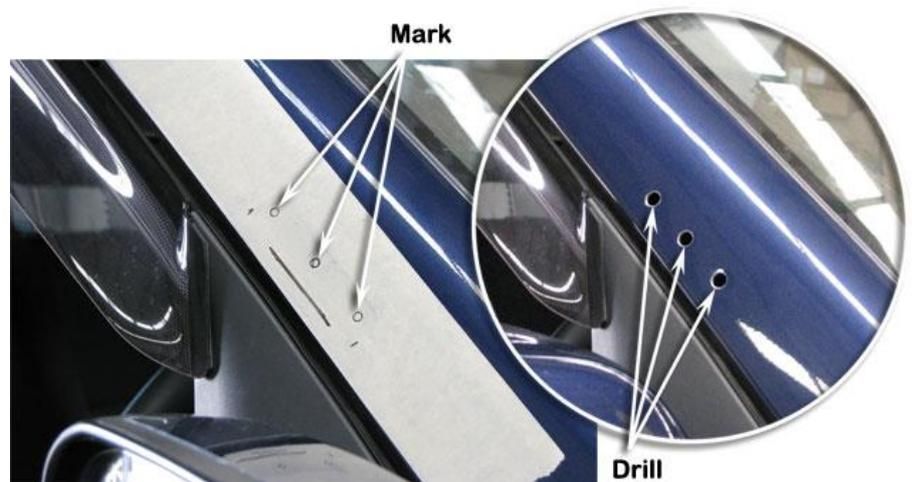
**NOTE: Extreme care must be taken when drilling the A-Pillar panel. The internal A-Pillar reinforcement can deflect drill bit.**
