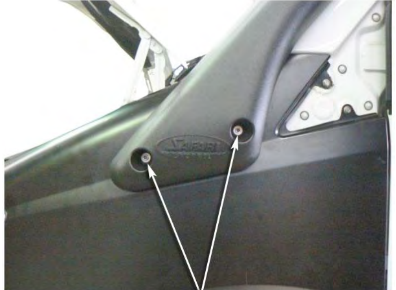
6mm Body Washers & M6 Socket Head Bolts
