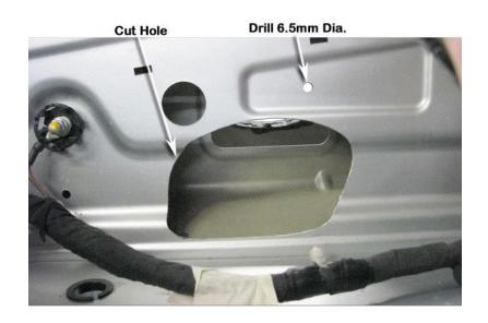
Re-install the wiring loom to the front and relocated mounting hole position, reinstall the coolant by-pass to the standard mounting positions as shown.
