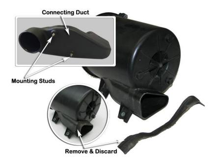
Install the connecting duct to the inner guard panel, fasten into position through the standard inner guard panel holes with 5.0mm body washers (item 14) and 5.0mm nyloc nuts (item 15) as shown.
