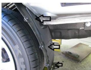
Remove x3 screws from front face of wheel
