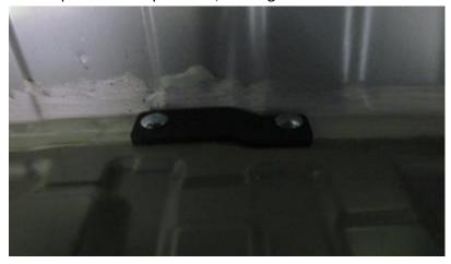
Bracket to be bolted to tab underneath towbar using the bolts provided then using the x1
