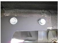
Holes x2 in centre plate are to be drilled through to boot using an 11mm drill bit.
