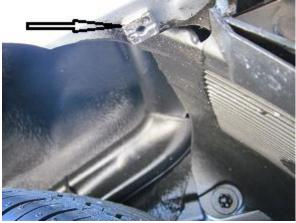
Remove x1 screw from top of wheel arch
