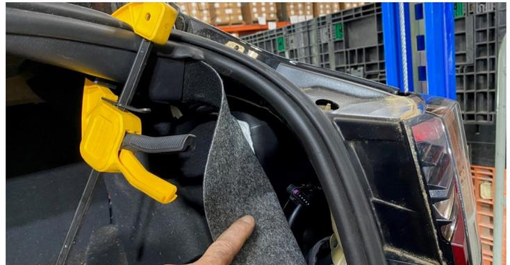
3. **2017-2023 Only:** Unplug the wiring harnesses from the taillights. Locate (2) nuts securing the taillights to the vehicle on either side of the trunk and remove.
